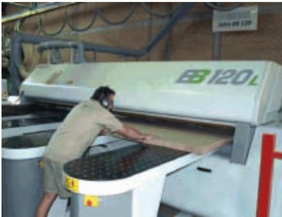
Sawing: - using a beam saw, CNC or dimensional panel saw.
